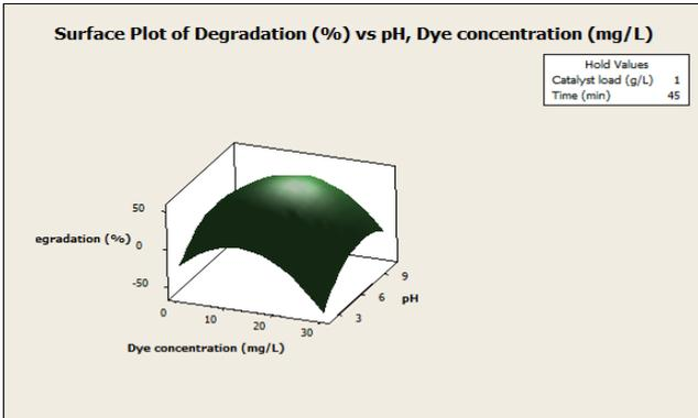
**Fig. 16:** Surface plot of % degradation versus pH and dye concentration
