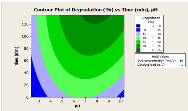
Fig. 6: Contour plot of % degradation versus time, pH
