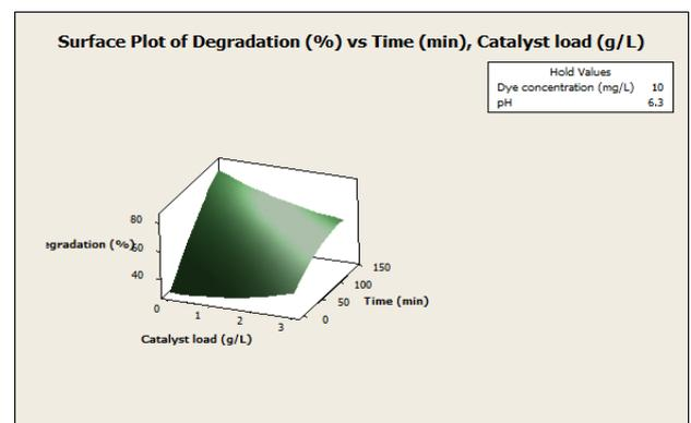
**Fig. 13:** Surface plot of % degradation versus time and catalyst
