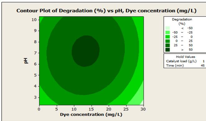
**Fig. 10:** Contour plot of % degradation versus pH, dye concentration
