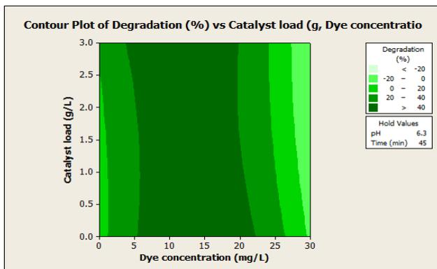
**Fig. 11:** Contour plot of % degradation versus catalyst load and dye concentration
