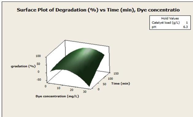
**Fig. 15:** Surface plot of % degradation versus time and dye concentration
