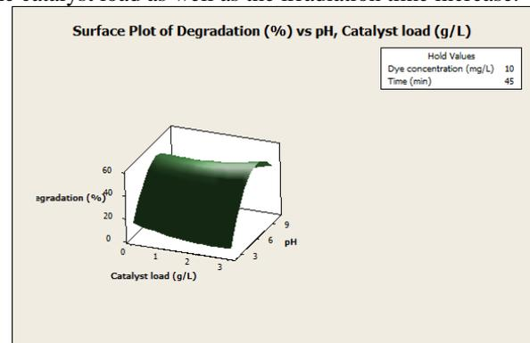
**Fig. 14:** Surface plot of % degradation versus pH and catalyst load
