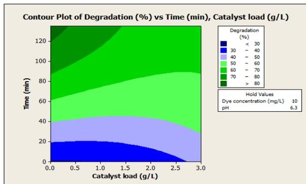
Fig. 7: Contour plot of % degradation versus time and catalyst load
