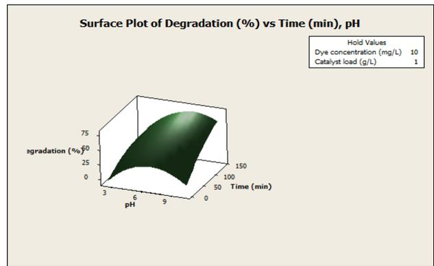
**Fig. 12:** Surface plot of % degradation versus time and pH
