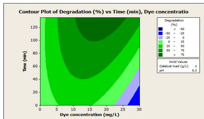
Fig. 9: Contour plot of % degradation versus time and dye concentration
