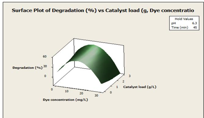
**Fig. 17:** Surface plot of % degradation versus catalyst load and dye concentration
