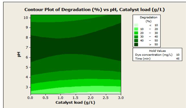
Fig. 8: Contour plot of % degradation versus pH and catalyst load
